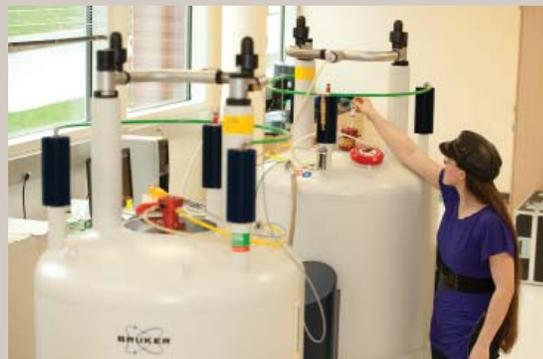
Additionally, two new 400 MHz NMR's were purchased for more routine spectroscopic needs. (1) Bruker DPX-400, a 2-channel spectrometer with a 5mm Broadband Observe (including 19F) probe with z-axis gradient. This spectrometer is currently running Topspin 2.1 software. (2) Bruker DPX-400, a 2 channel spectrometer with both 5mm Broadband Observe and a 5mm Broadband Inverse probe both with z-axis gradient. This spectrometer is currently running Topspin 1.3 software.
