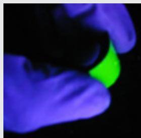
High-temperature, light-emitting ceramic film deposited onto a flexible plastic substrate, p. 16
